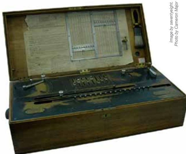
This Millionaire calculating machine was used in the compilation of 1911 census results
